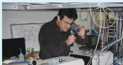
Prof. Kinoshita is checking optical alignment through an Infrared viewer.
